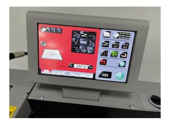
A user friendly SmartScreen panel enables adjustments to 0.1mm on the fly if the fold plates or delivery roller needs to be moved. Within this SmartScreen panel are a counter and batching facility which are standard features. A further feature of the sophisticated SmartScreen is the ability to memorise and store repeated jobs in the alpha numeric memory which can then be retrieved within seconds.
