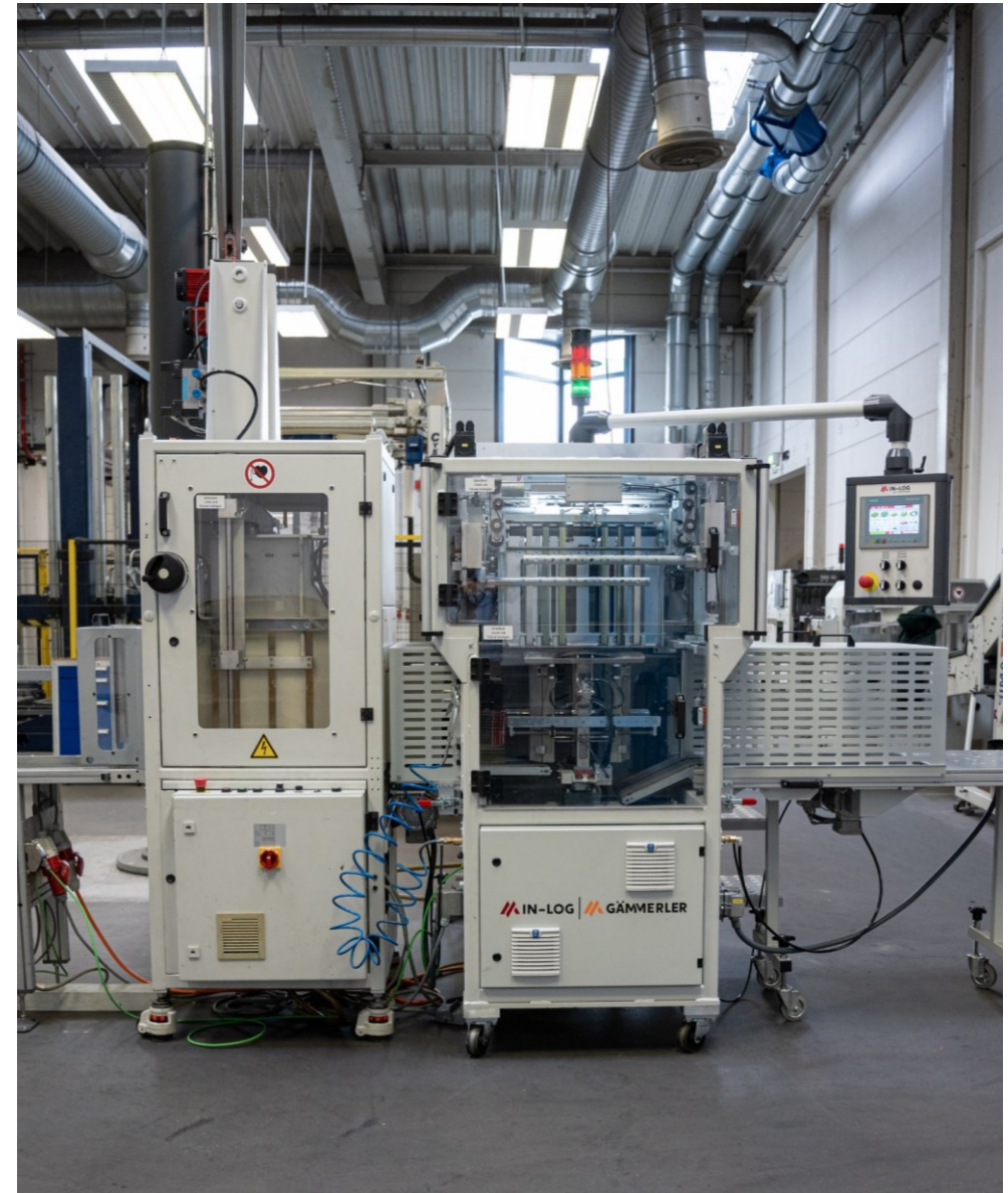
▲ Teamwork – new CS/3160 lift stacker closed coupled with the existing VM 500 blocking unit from Gämmerler
