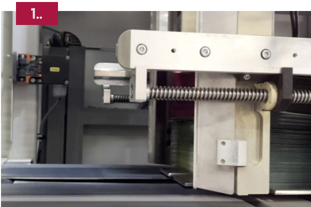
1.. ▲ Delivery belt pivots up to receive bundle
