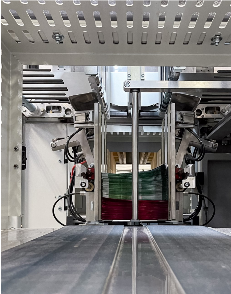
▲ Heavy duty turntable with electrical size adjustment.
