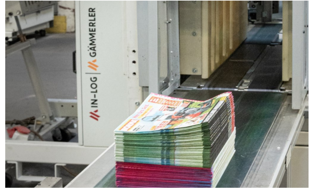
▲ Closed coupled blocking unit stabilizes the bundle
