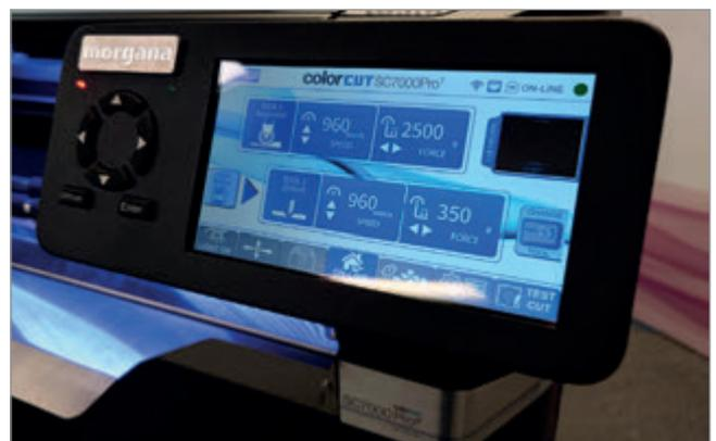
The 7 inch immersive touch screen control panel can pivot to suit the angle desired by the operator.
