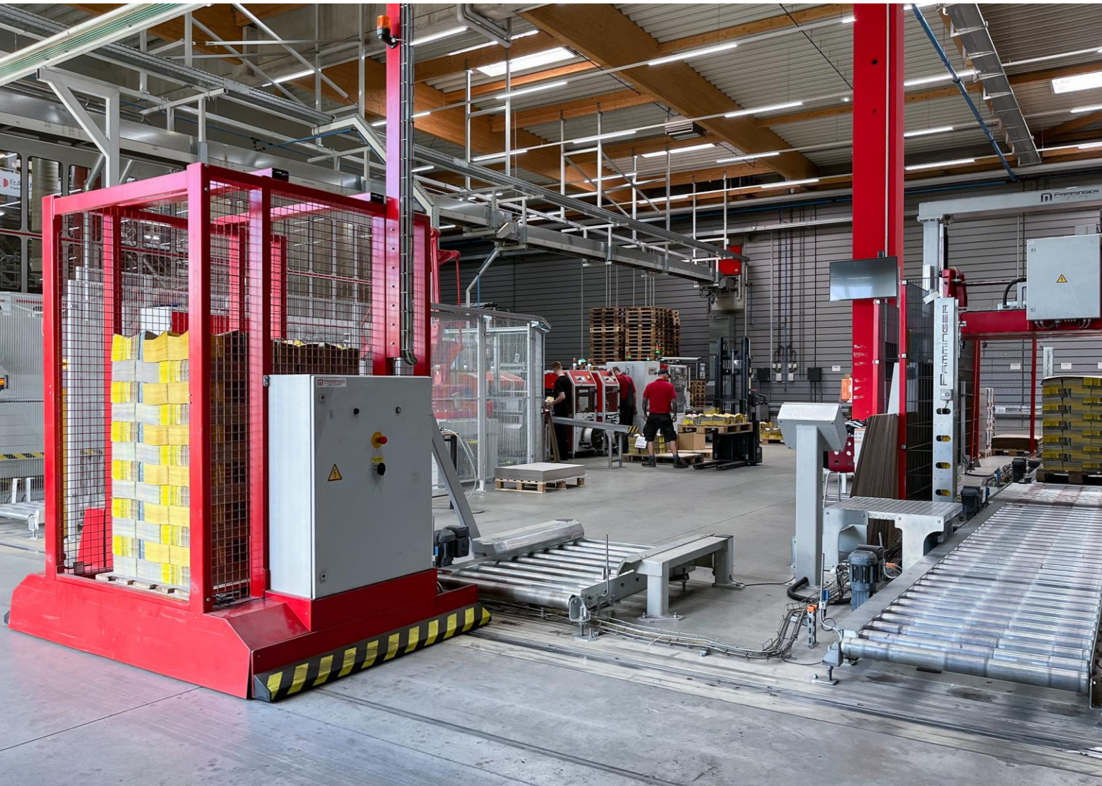
▲ The shuttle delivers the full pallets onto an automatic line for pallet strapping and stretch wrapping.
