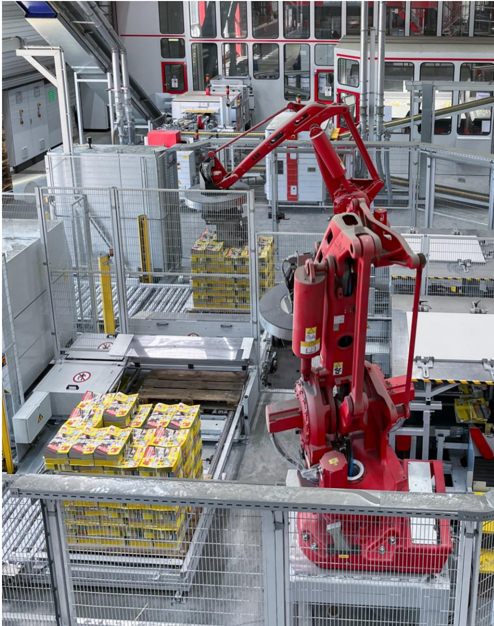
▲ The palletizing area integrates two robotic arms, each of them handling one line.
