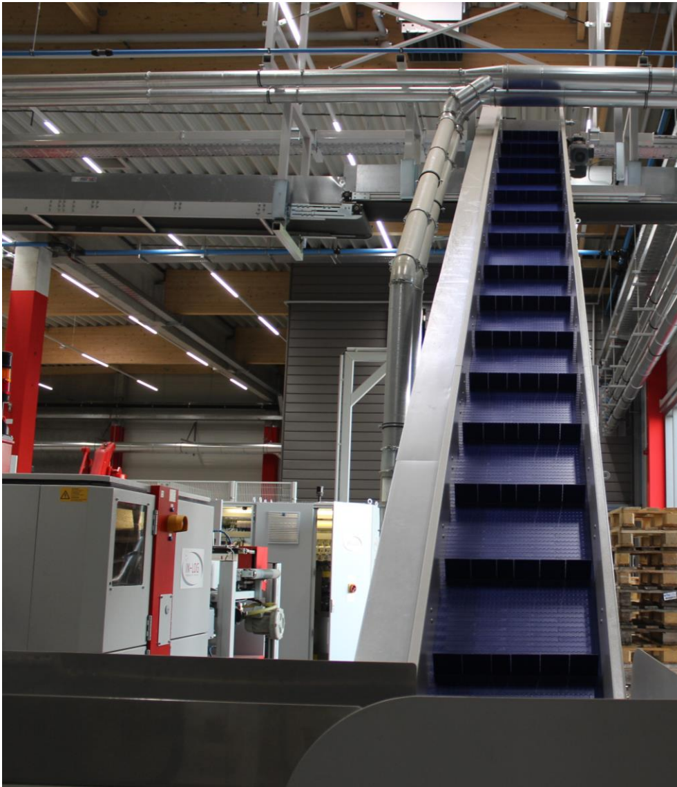
▲ The incline conveyor dumps the waste from the 96p press onto a central overhead waste conveyor which serves several presses.
