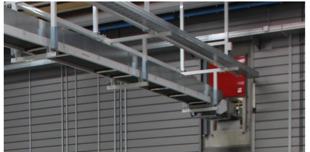
▲ One waste conveyor collects the waste from different presses and brings it to a central waste bin outside the building
