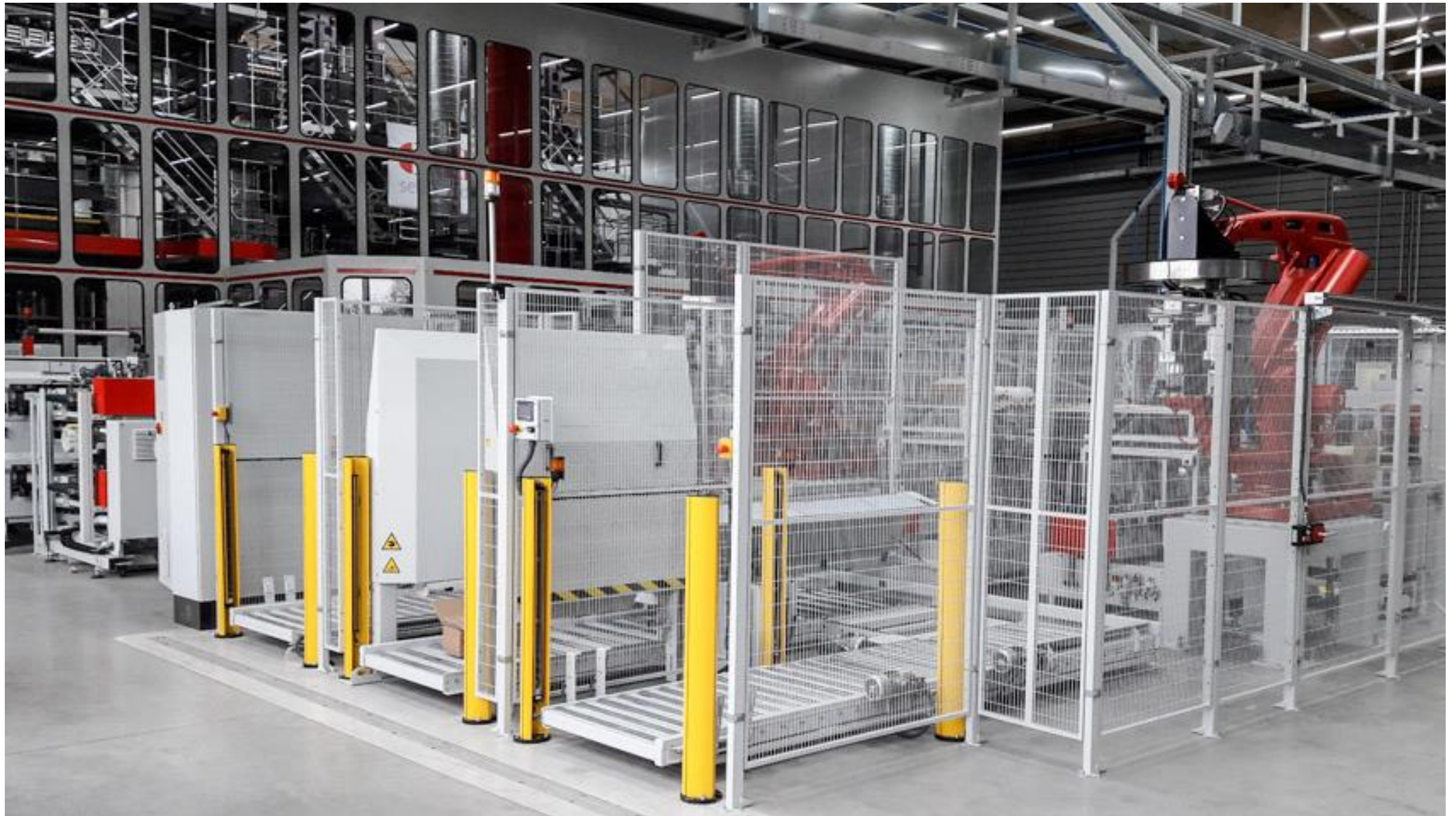
▲ The palletizing area – fully automated, with two robots, including empty & full pallet conveying.
