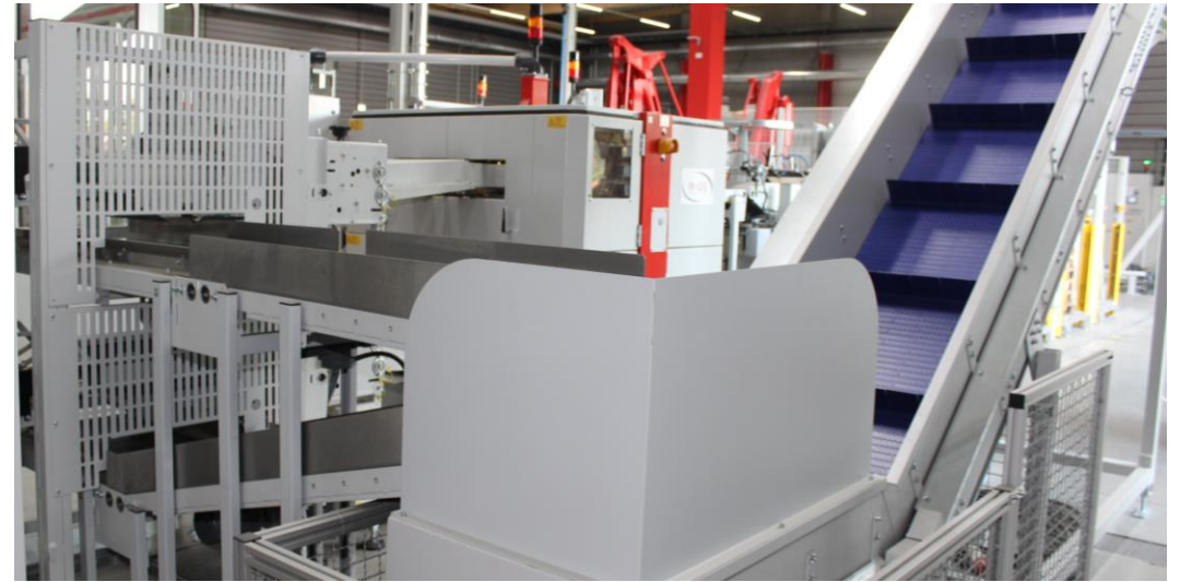
▲ Waste from the conveying lines goes onto an incline conveyor
