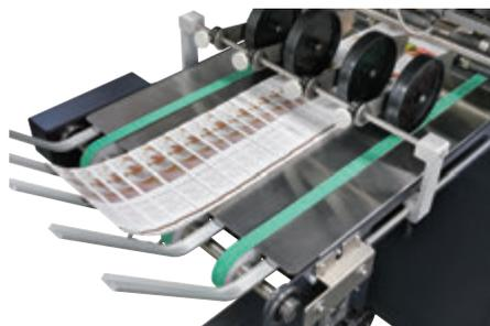
The standard delivery conveyor SCV-406 is appropriate for space saving system configurations. Conveyor height and delivery speed can be easily adjusted to the proper sheet delivery. More delivery unit options such as the knife unit and stacker are also available depending on your needs.
