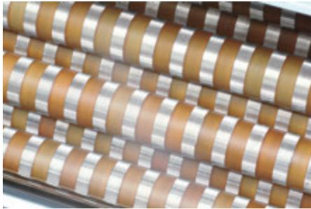
Unique design and precision manufacturing insures folding accuracy and long roller life. Soft or hard urethane rollers are available depending upon folding requirements.
