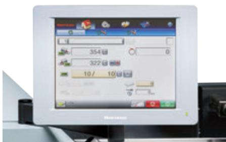
The 12.1 inch color touch-screen is icon-based for user-friendly operation. Each section is automatically set by inputting sheet size and fold pattern. Roller gaps can be adjusted by 5 µm (0.005 mm) and the buckle stopper can be adjusted by 0.1 mm / 0.005" at the touchscreen. Up to 200 job settings can be stored in job memory.
