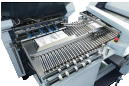
Auto adjusting conveyor and guides with conical drive rollers efficiently transfers even complex folded sheets to the second fold section.
