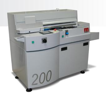
Another feature of this applicator is it can be cleaned and sealed automatically from the touch screen allowing for minimum glue wastage.
